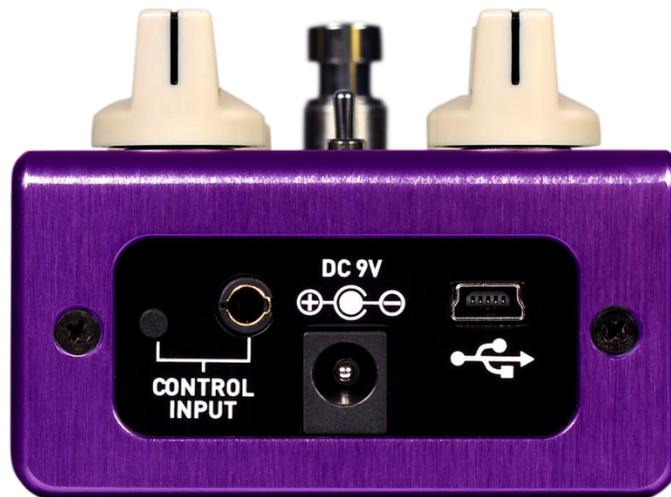
The CONTROL INPUT port opens a variety of external control options, allowing for direct control over many of the Spectrum’s parameters. It is an input for the, Source Audio Tap Switch, Source Audio Dual Expression Pedal, or a data port for the Neuro Hub.
