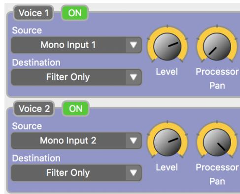
The Spectrum features two standard Voices. Each Voice can receive signal from either Mono Input 1, Mono Input 2, or Stereo Input Mix. Both Voice modules feature the same control set.
